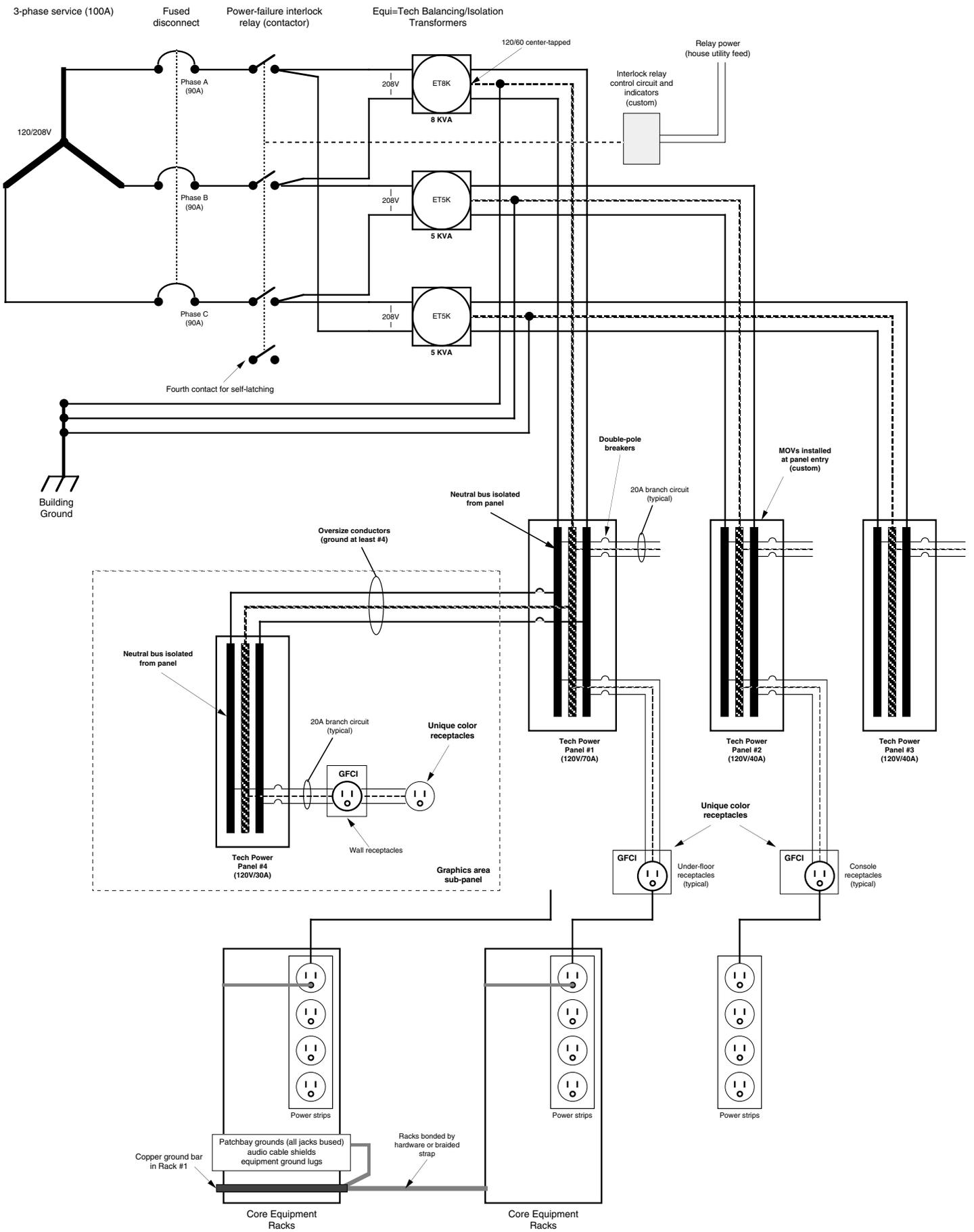
**Fig. 1 Power/Grounding Conceptual Block Diagram**
