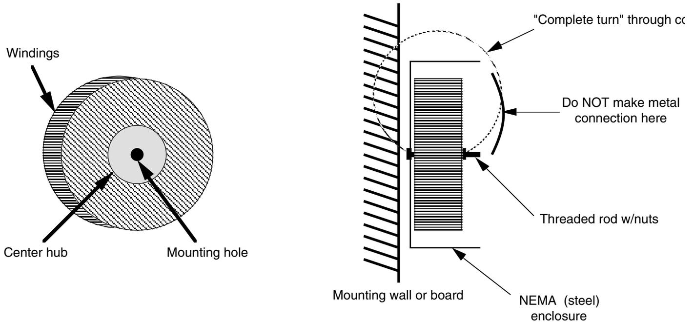
**Fig. 2 Toroidal Transformer Mounting**
