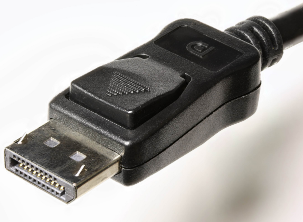
DisplayPort Computer video & HDTV With audio Latching connector!
