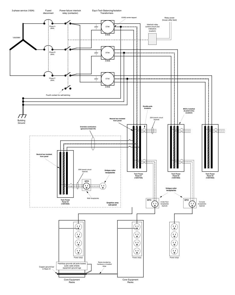
Fig. 1 Power/Grounding Conceptual Block Diagram Fast Cuts, Inc. Washington, DC
